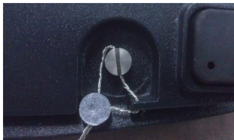
Locked with Wire Seal
